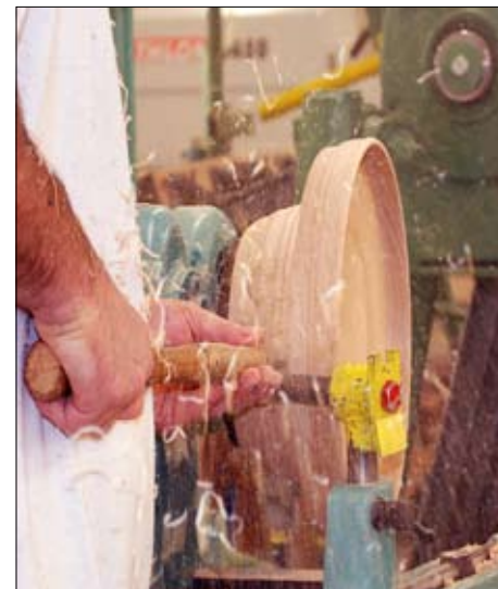
Above, like Tass Jansen, Rick Hobbs , left, and Tony Whisnant , both Correction Enterprises supervisors, test a couple of chairs for their restfulness. Below, slivers of wood fly as an inmate sculpts a wooden bowl on a lathe. All of the wood products were once scrap pallet wood.
