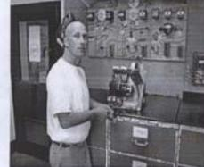
Student putting the finishing touches on a project that controls a reversible motor complete with indicator lights and safety interlocks.
